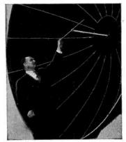
Research in microwaves and electron tubes at RCA Laboratories led to the development by the RCA Victor Division of this automatic radio relay system. Here is a close-up view of a microwave reflector. This system also holds great promise of linking television stations into networks.
