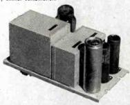
The Type 201-B Rectifier supplies plate and filament power for the Langevin Types 102, 106, 111 and similar amplifiers from a 105-125 volt, 50-60 cycle AC source. The ripple voltage of the 201-B Rectifier is 0.04% at full power output 75MA and 0.02% at a drain of 30 milliamperes.
